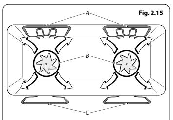
A – Broiler elements, B – Convection element, C – Base heat elements
