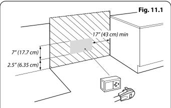
The dimensions shown are correct when the range is set to its lowest position
