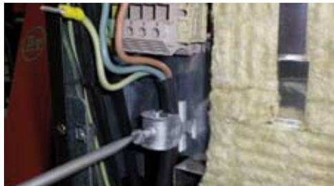
5. Install the power cord: attach the wires to the terminal block as follows:
