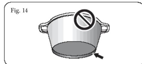
Simmering aids, such as asbestos or mesh mats, are NOT recommended. They will reduce burner performance and could damage the grates (Fig. 15).
