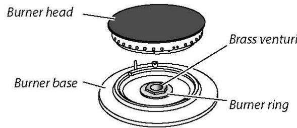
Orifices of gas burner are replaced by means of this sequence:
