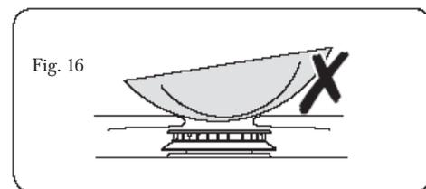
The minimum pan diameter recommended is 12 cm for the outer burners and 16 cm for the center burner.
