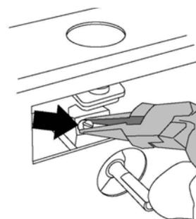
4. Using a pair of long nose pliers carefully remove the bypass screw.
