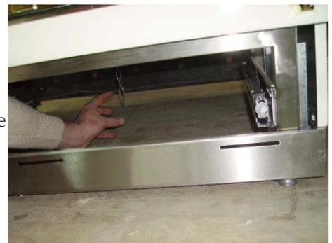
9. Attach the chain to the stud with the help of the snap hook.
