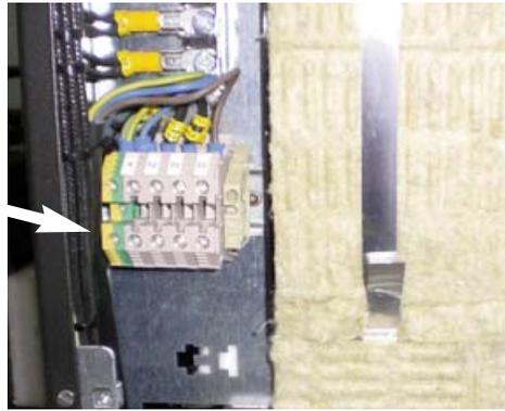
3. The appliance is shipped with a strain relief device to secure power cord. Insert the power cord through the strain relief and tighten it.
