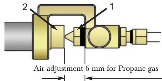
1. Screw the adjusting cone (2) and insert it into the mixing tube in order to free sufficient space for unscrewing the orifice.
